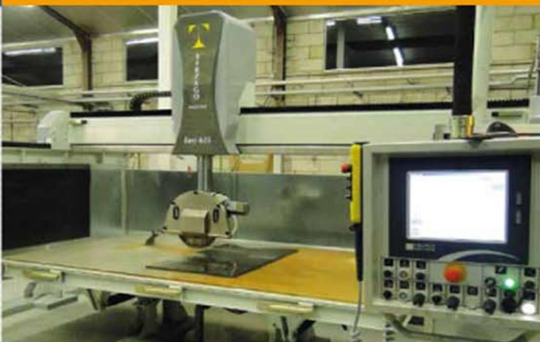
5 AXIS CNC MILLING AND CUTTING BRIDGE SAW
