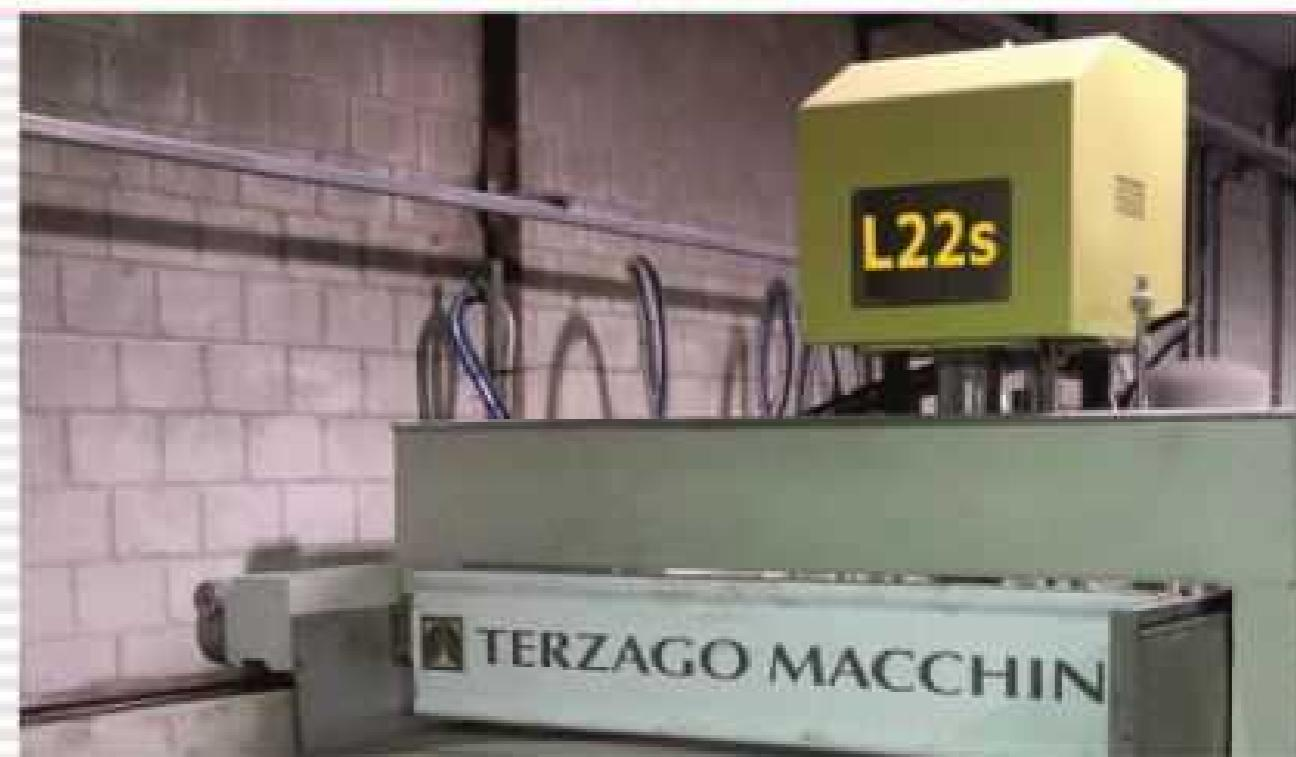
POLISHING-CALIBRATING MACHINE FOR MARBLE AND GRANITE
